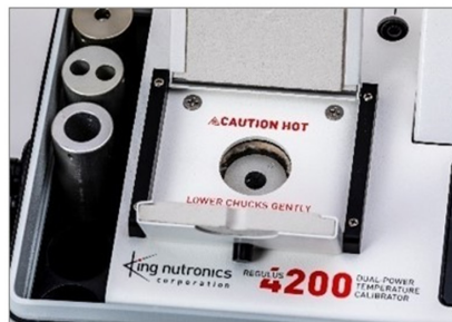
Figure 3-1 Inserting an Adapter Chuck and a UUT
