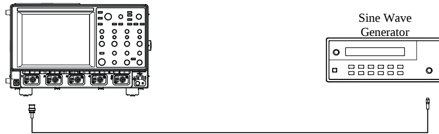
Figure 5-3 : 50Ω Bandwidth Equipment Setup
