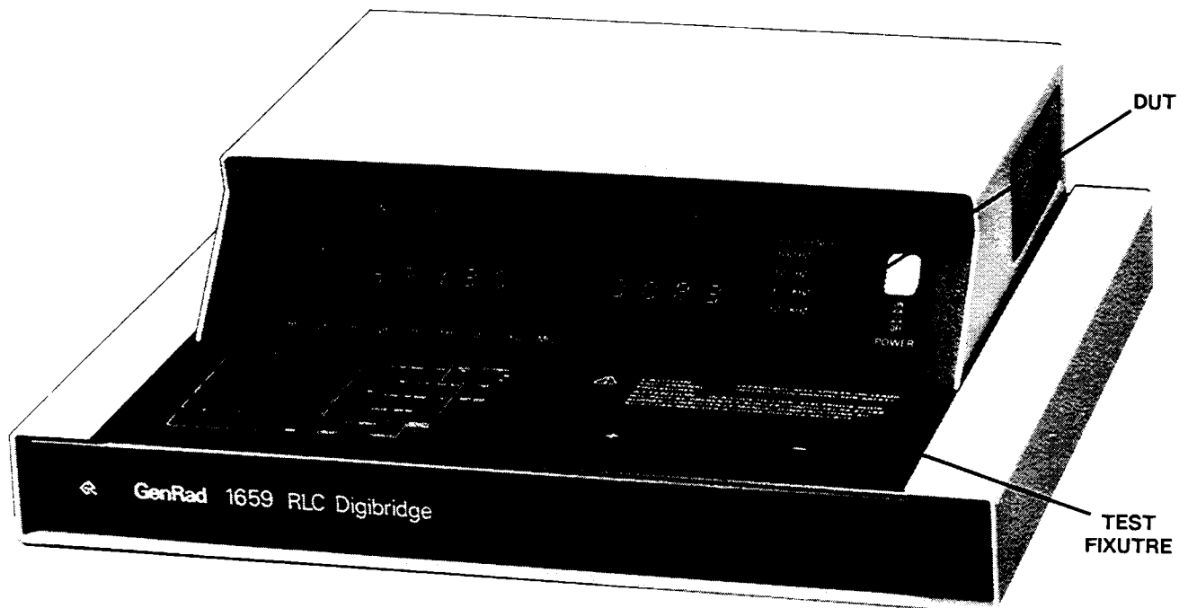
Figure 3-1. A radial-lead DUT is inserted into a Digibridge test fixture.
