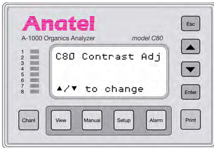
Fig 4-4 : C80 Contrast Adjustment Screen
