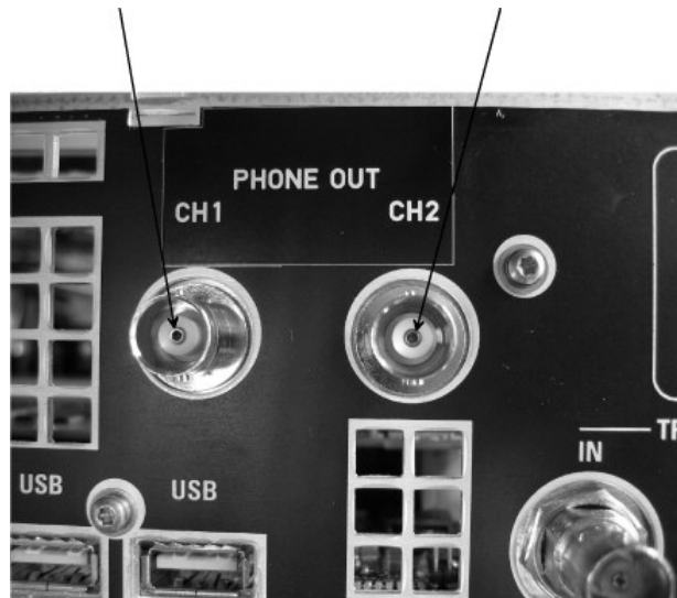
Fig. 4-3 Position of female BNC connectors and adhesive label on the rear panel
