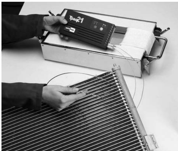
Thermocouple probes being attached to a radiator test piece.
