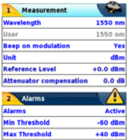
Fig. 13 Configuration of power measurement
