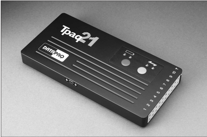
10-channel Tpaq21 logger, showing LEDs and stop/start buttons (upper surface), communications port (front edge) and thermocouple and transmitter aerial sockets (right).
