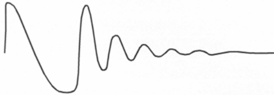
Fig 6.1: Example of a "ringing" wave pattern resulting from Surge Testing
