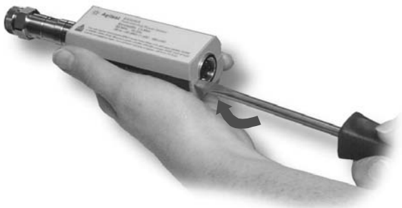
Figure 12 Removing Power Sensor Shell
