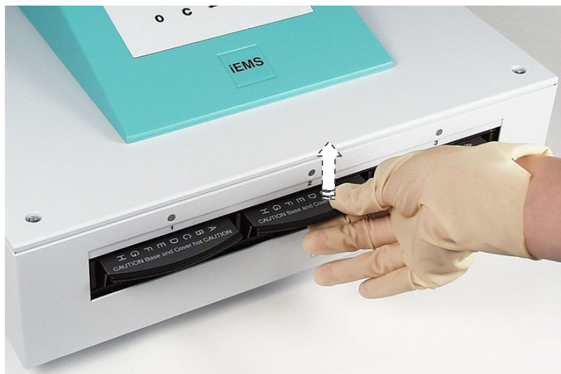
Fig. 6.5 Removing the microplate holder – lifting the handle
