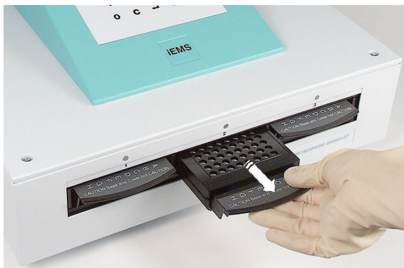
Fig. 6.6 Removing the microplate holder – pulling the holder out
