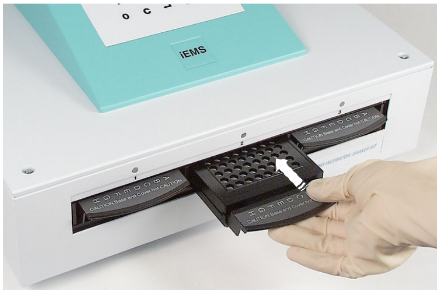
Fig. 6.3 Inserting the thermal microplate holder into a slot
