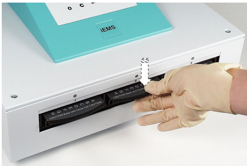
Fig. 6.4 Pushing down the microplate holder to latch it properly
