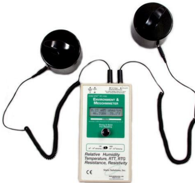
Figure 4 - Ohm - Stat RT-1000 Point to Point (RTT) test.
