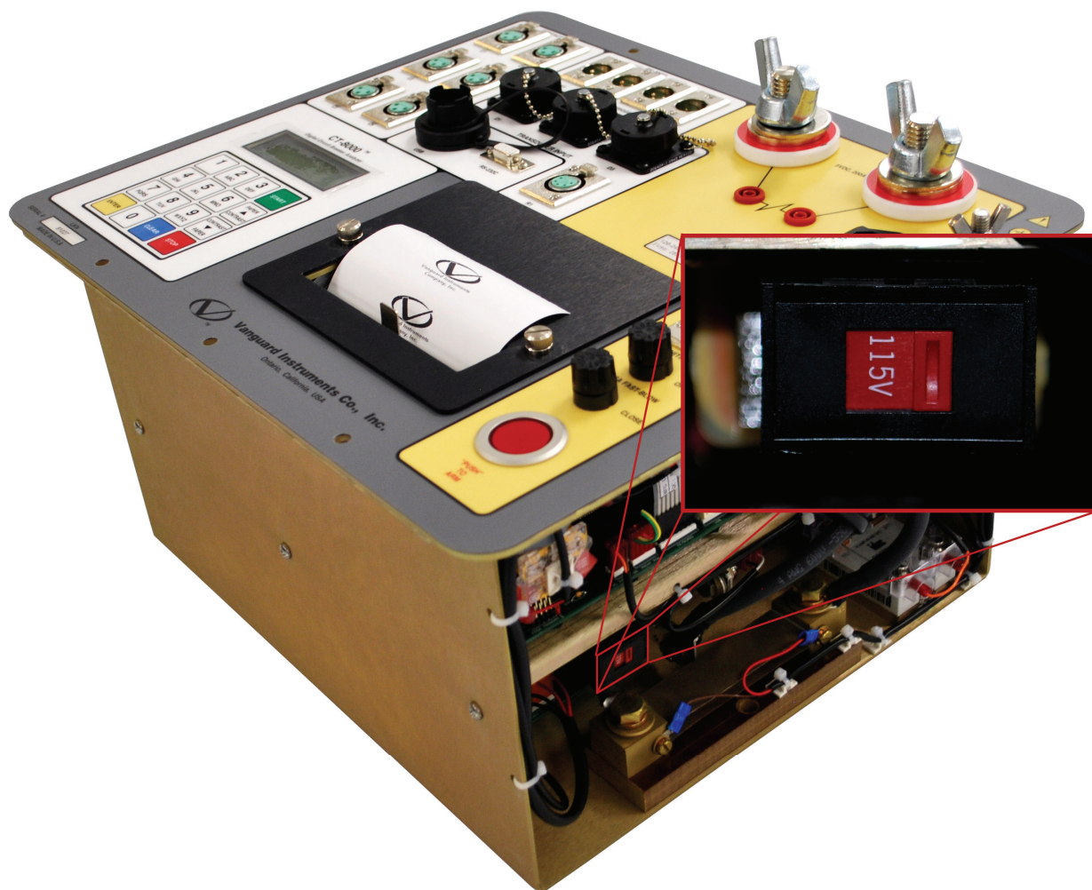
Figure 2. CT-8000 Operating Voltage Setting Switch
