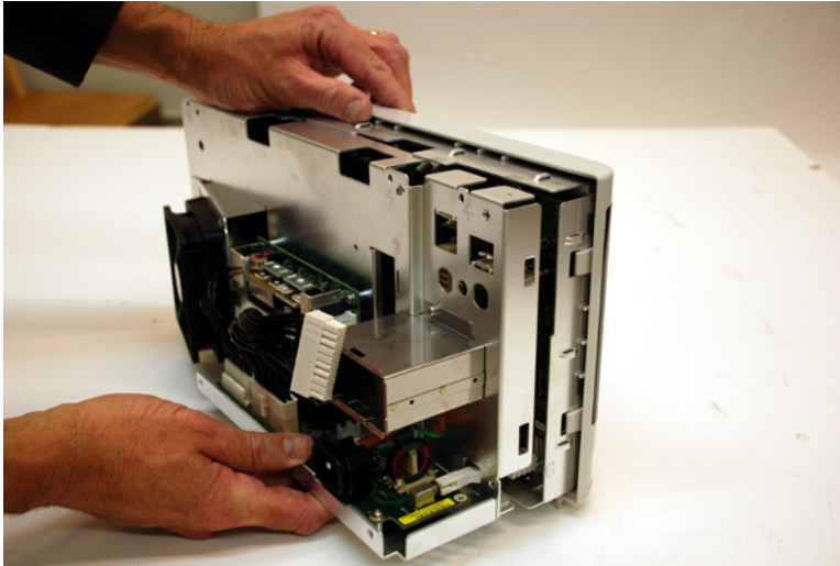
Figure 35 Separating the rear and front decks
