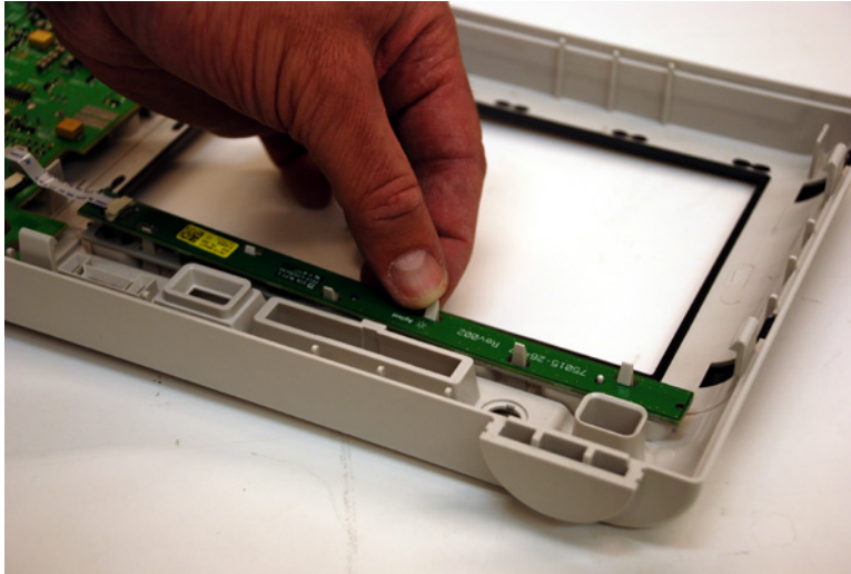
Figure 50 Unclip the softkey board from the bezel
