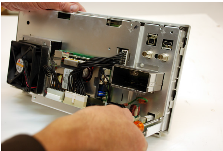
Figure 29 Removing the bottom right rear deck screw
