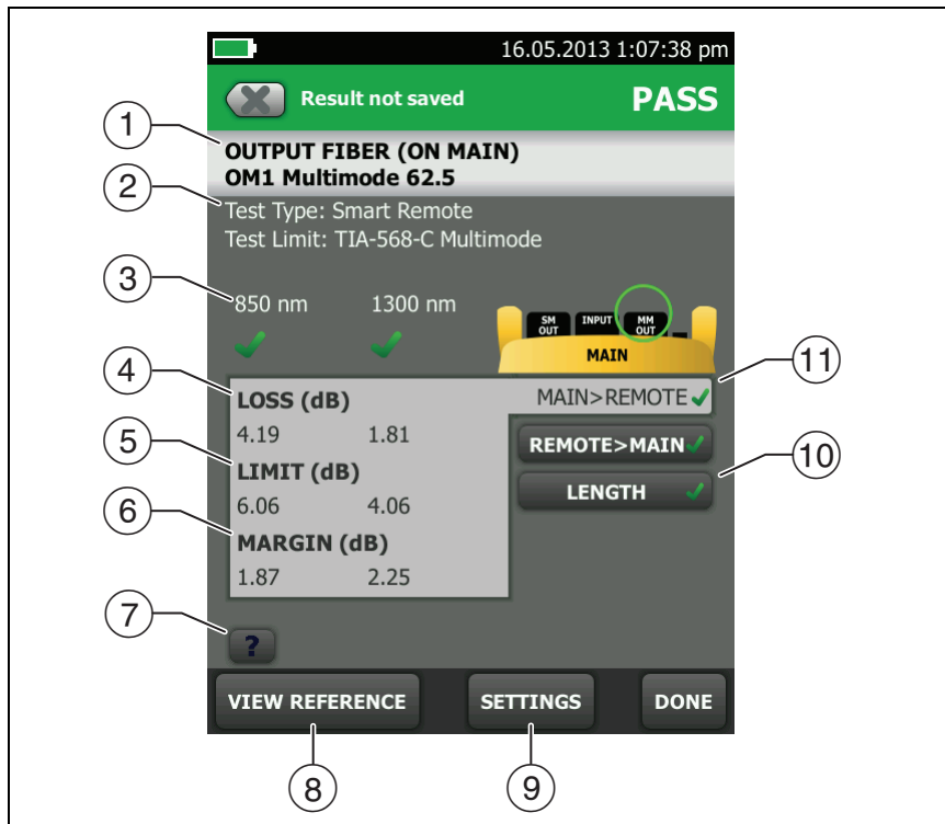
Figure 114. Detailed Result for Smart Remote Mode (Unsaved Bi-directional Results Shown)
