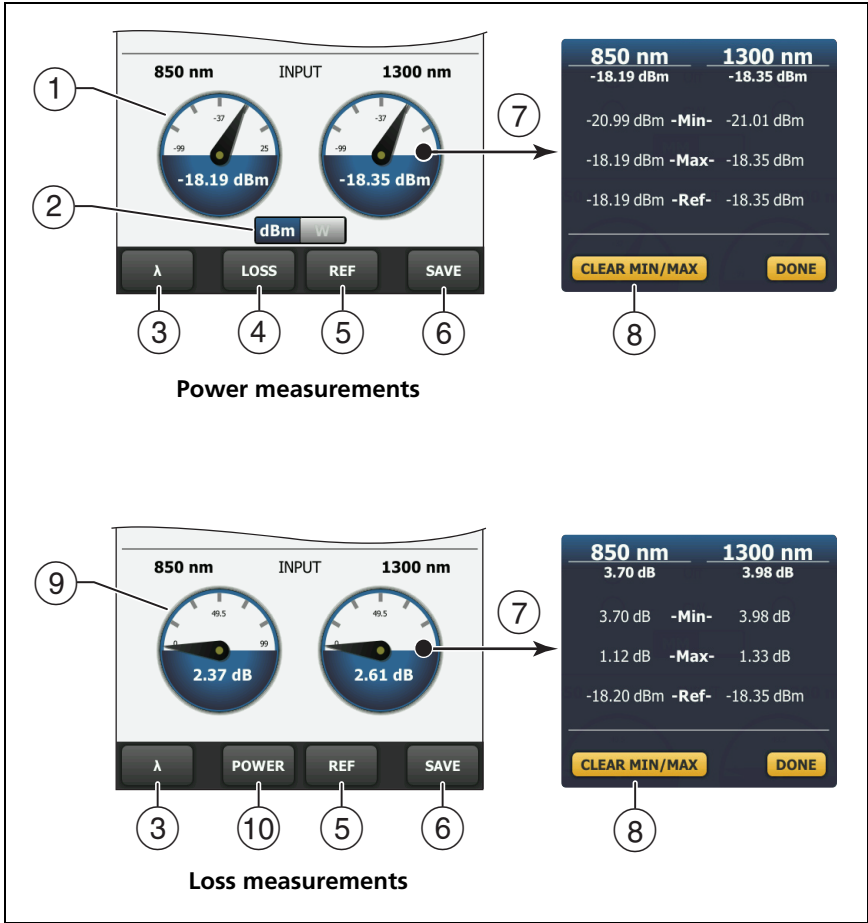
Figure 127. Power Meter Measurements and Controls
