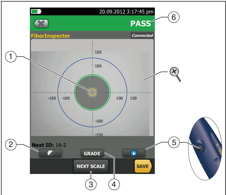
Figure 100. FiberInspector Image with Manual Grading Selected
