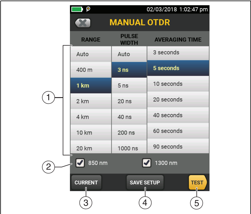
Figure 151. Manual OTDR Screen for Quick Changes to Test Settings
