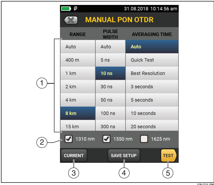
Figure 176. Manual PON OTDR Screen for Quick Changes After a Test
