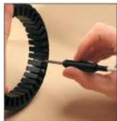
Fig. left: DUALSCOPE® MP20 with eddy current probe to measure coating thickness on NF metals.
