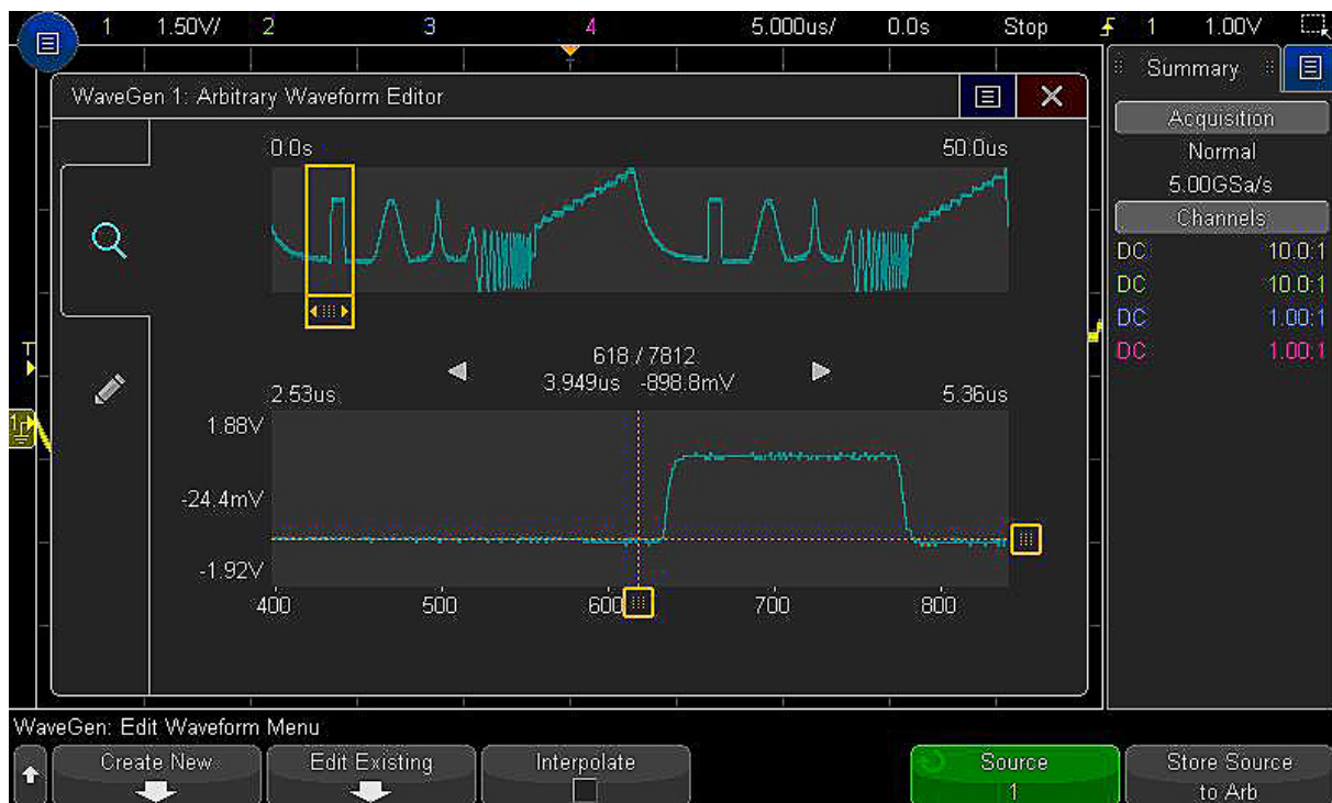
Figure 24. Optional arbitrary waveform generator provides easy access to stimulus. The integrated arbitrary waveform generator makes capturing, modifying and replaying signals simple.
