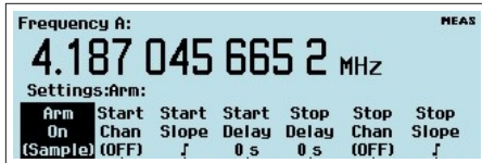
Fig. 2-15 CNT-91(R): Setting arming conditions.
