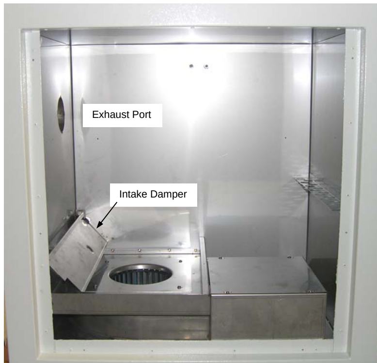
CONDITIONING PLENUM – INTAKE DAMPER FULLY OPEN
