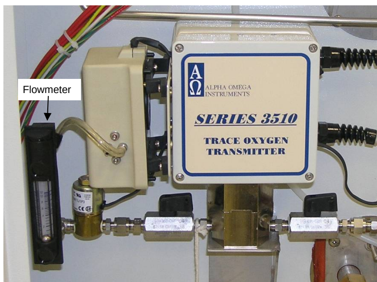
SERIES 3510 TRACE OXYGEN TRANSMITTER Series 2510 is similar in appearance
