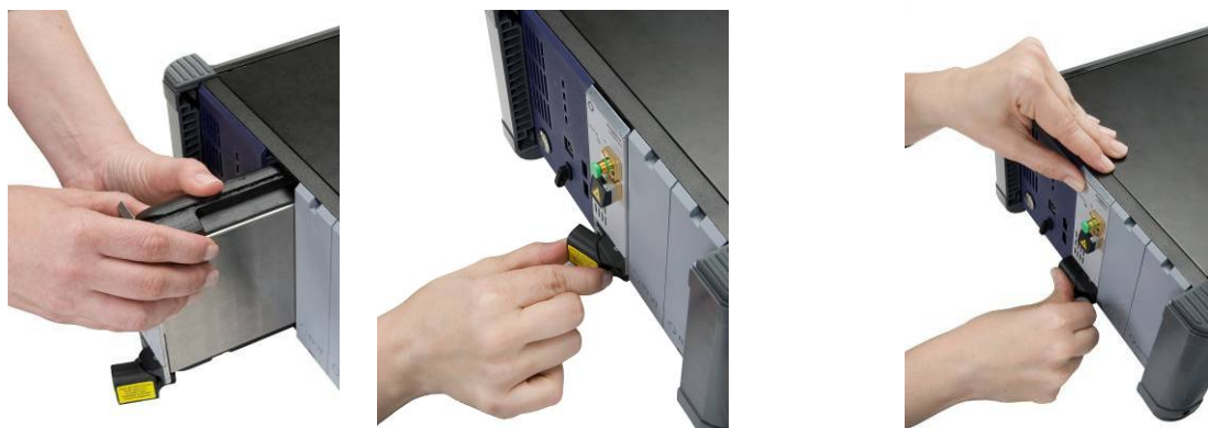
Figure 45: Inserting an Optical Module
