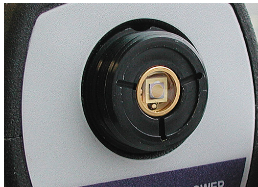
Figure 98: 2mm InGaAs General Purpose MAP Power Meter
