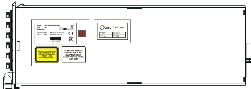
Figure 15: MAP-200 Cassette Labels, clockwise from left: Identifier label, RoHS label, Calibration label, FDA label and laser classification label
