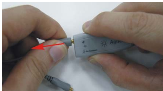
Figure 2-17 Pull the probe head straight out to disconnect it from the amplifier
