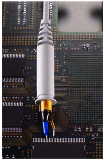
Figure 2-6 E2676A single-ended browser probe head
