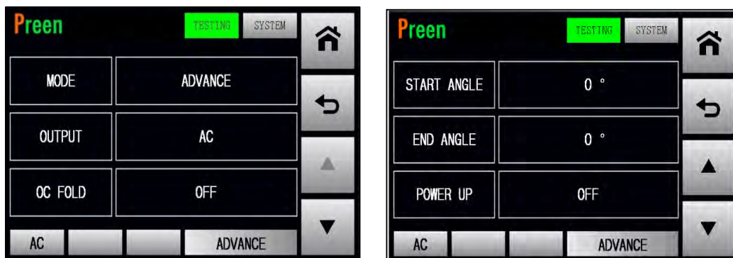
Figure 3.9 TESTING subpages 1 & 2 (ADVANCED mode)
