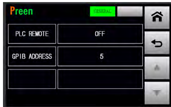
Figure 3.43 GENERAL subpage with the GPIB interface
