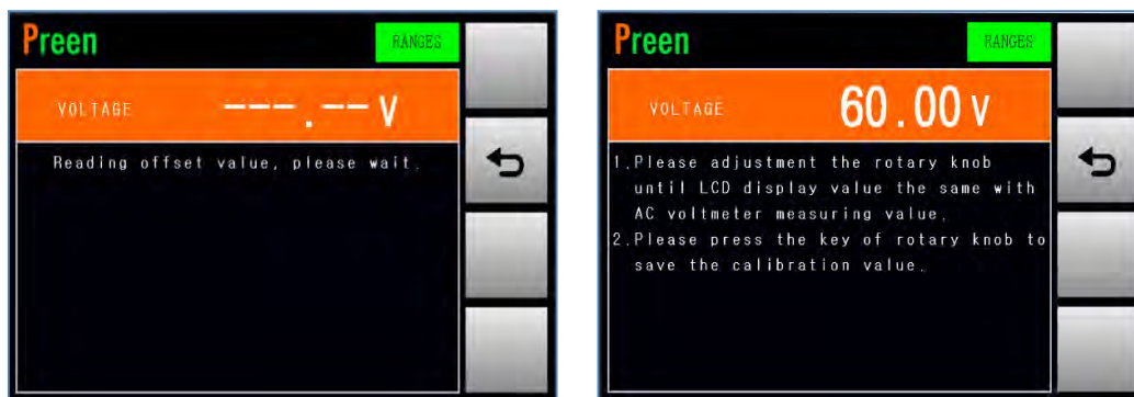
Figure 4.10 Enable the calibration of the HI-Range voltage 60V
