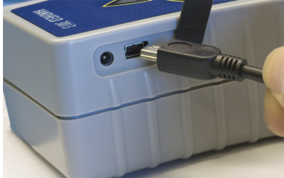
Figure 3-2 Connecting USB data communications cable
