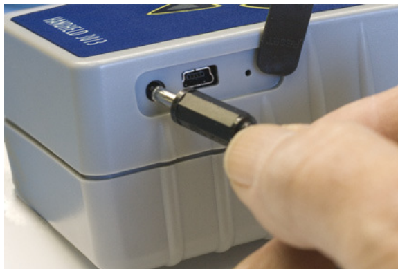
Figure 3-1 DC power plug
