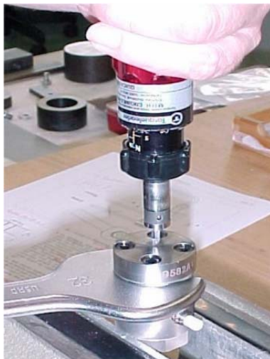
Fig. 8: Installing reaction torque sensor
