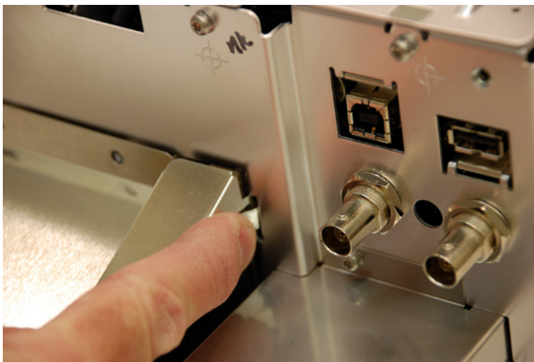
Figure 25 Unclipping the power supply shield right side
