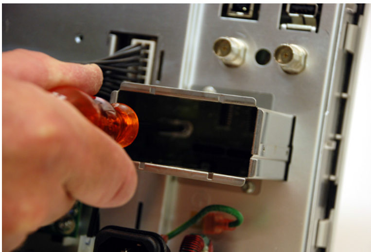
Figure 32 Removing the option module guide to acquisition board screw
