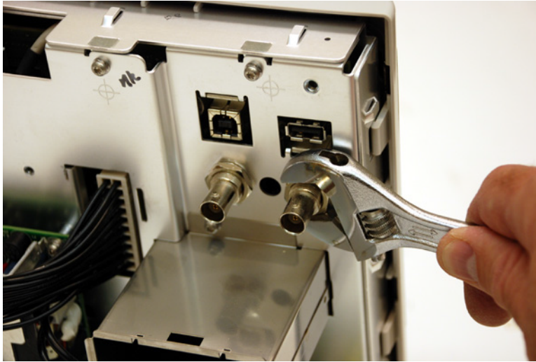
Figure 27 Removing the BNC nuts and washers
