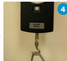
Apply Pull Force Apply a pulling force to the sample under test. Observe the load bargraph (fills from the center towards the “T”) and the Tensile Load Indicator (arrows). The main display will indicate the load being applied to the load sensor shaft using the fixture/adapter.
