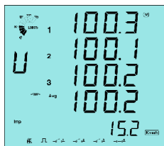
Fig 3.21 Inductive reactive energy
