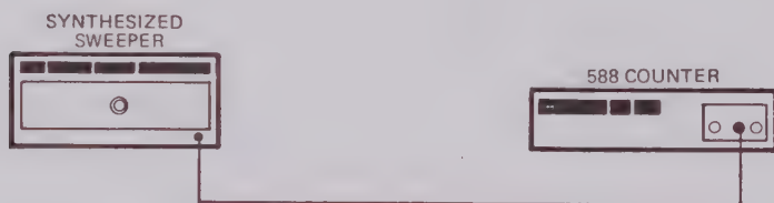
Figure 4-25. Band 2 Center Frequency Test Setup
