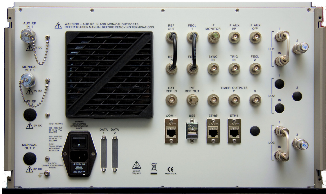
Figure 6-4 GSS8000-series single-output signal generator - Rear Panel
