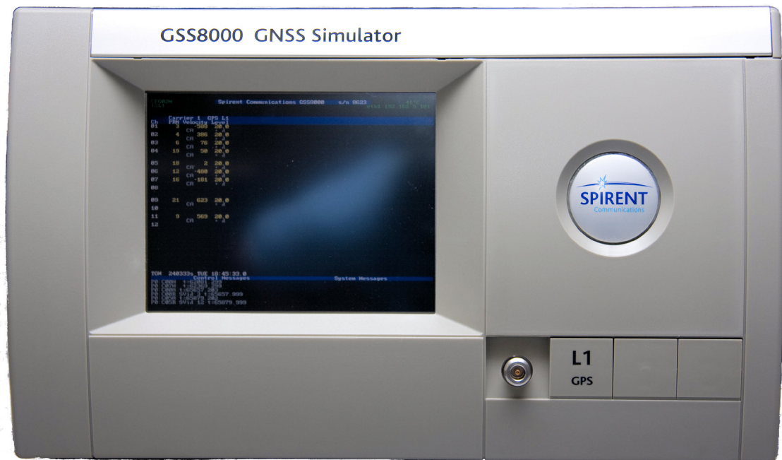
Figure 6-1 GSS8000-series single output signal generator - Front Panel
