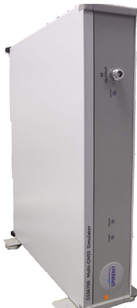
Figure 3-24 Vertically mounted GSS6700
