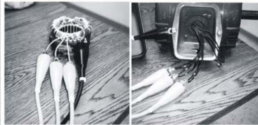
Fig 7-2: Tester/motor hookup example
