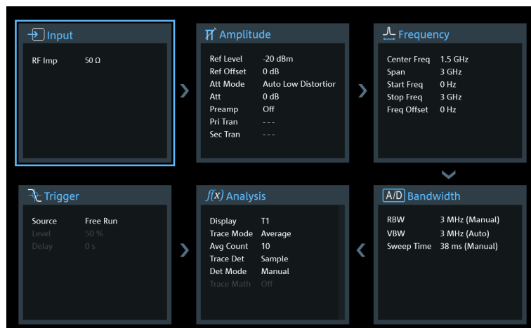
Figure 15-1: Configuration overview in the spectrum application
