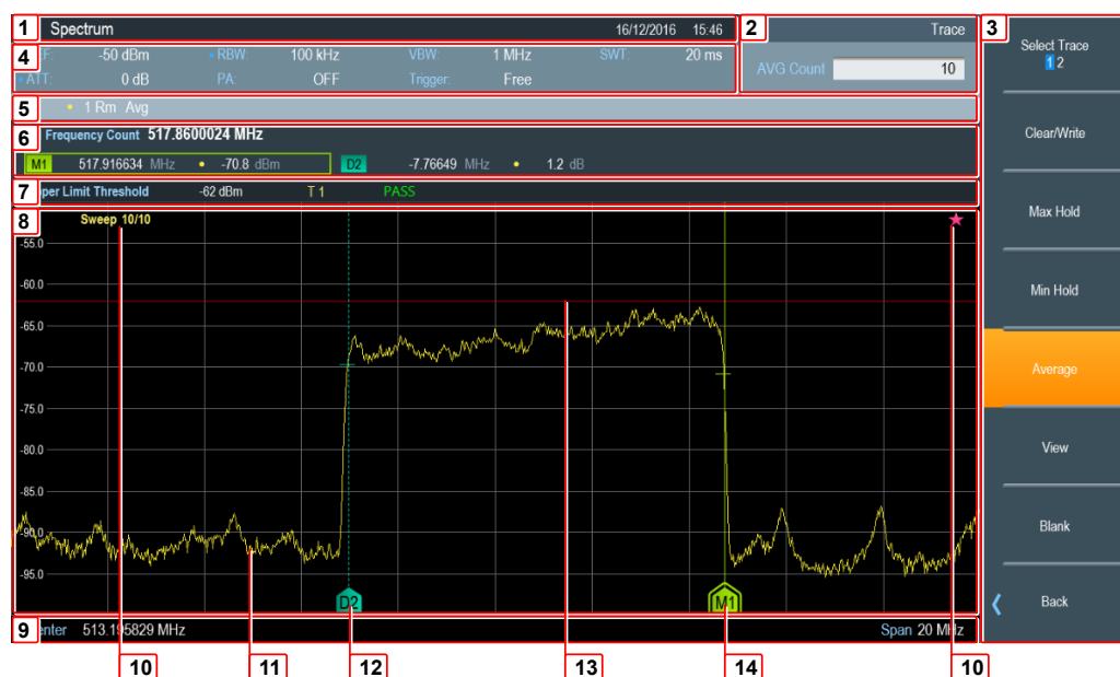
Figure 6-7: Screen layout in the spectrum application
