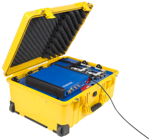
Figure 5-2: Connecting FRANEO 800 to the computer by using the delivered USB 2.0 A/B cable
