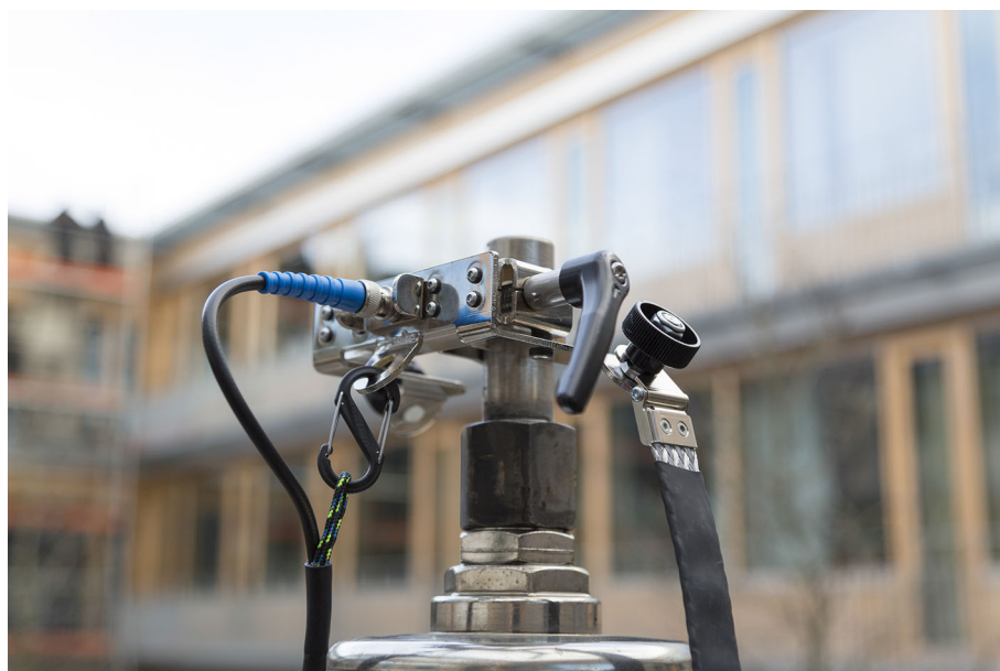
Figure 5-7: Connecting the blue coaxial cable to the bushing clamp by using the mechanism for relieving the pressure on the BNC shield
