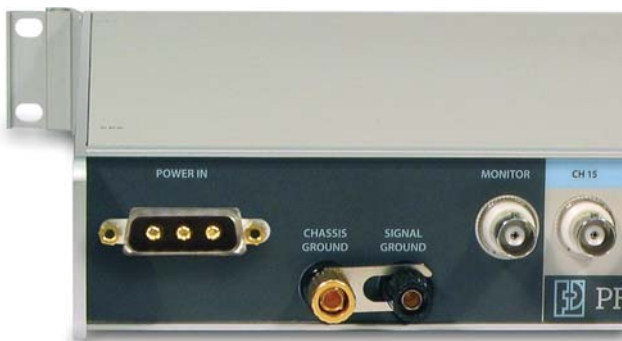
Figure 2.8 Power Entry, Ground Binding Posts and MONITOR Output Connector
