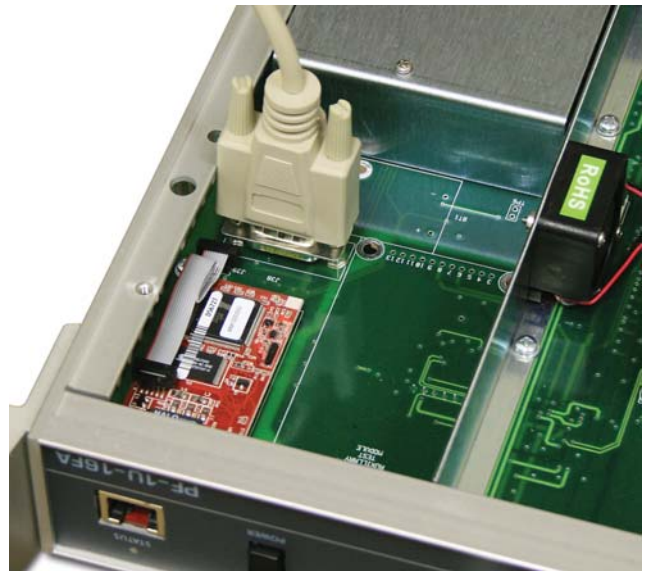
Figure 2.11 Connection to Programming Port
