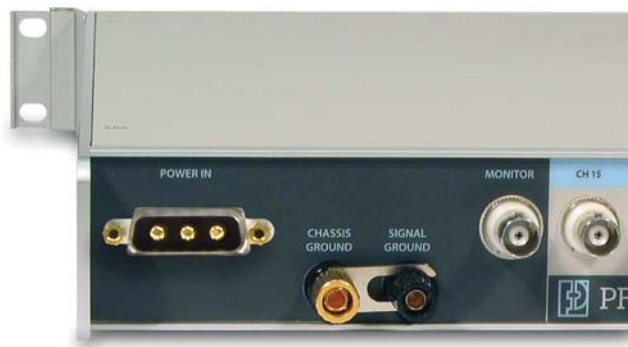
Figure 1.3 Power Entry, Ground Binding Posts and MONITOR Output Connector
