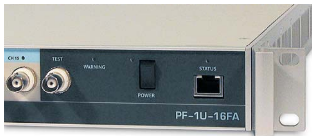
Figure 2.3 Front Panel Ethernet Connector
