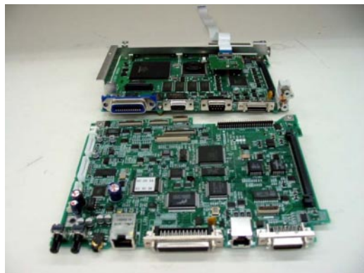
CPU board separated from the I/O board.
