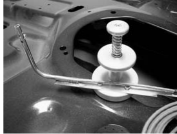
Aluminum automotive probes in use – surface probe (left) and air probe (right).
