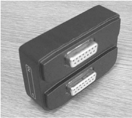
Dual Interface Block, showing connectors for two Transducer Interfaces.
