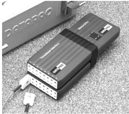
Dual Interface Block in use, connected to two Transducer Interfaces and a MemoryPaq.
