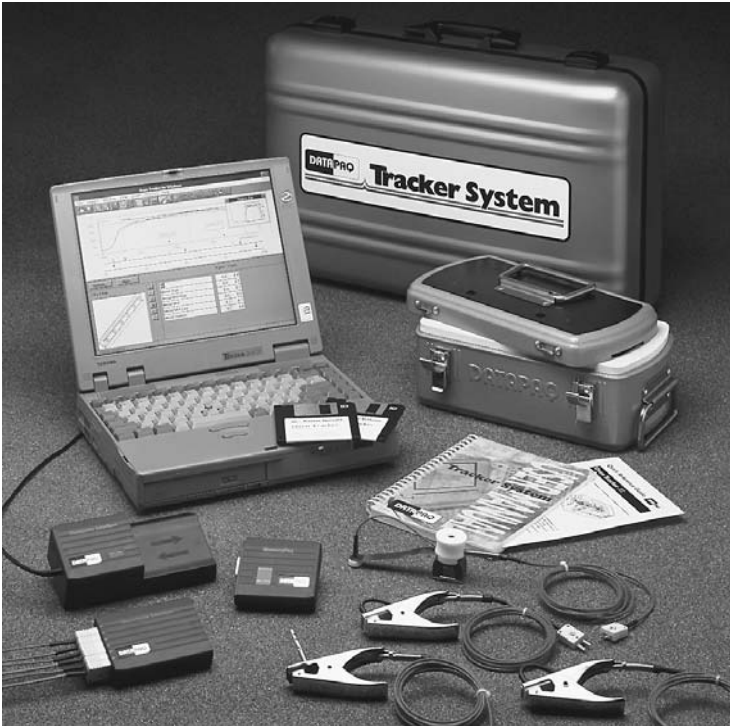
Components of the Oven Tracker XL system, together with a laptop PC (the charger is not shown).
