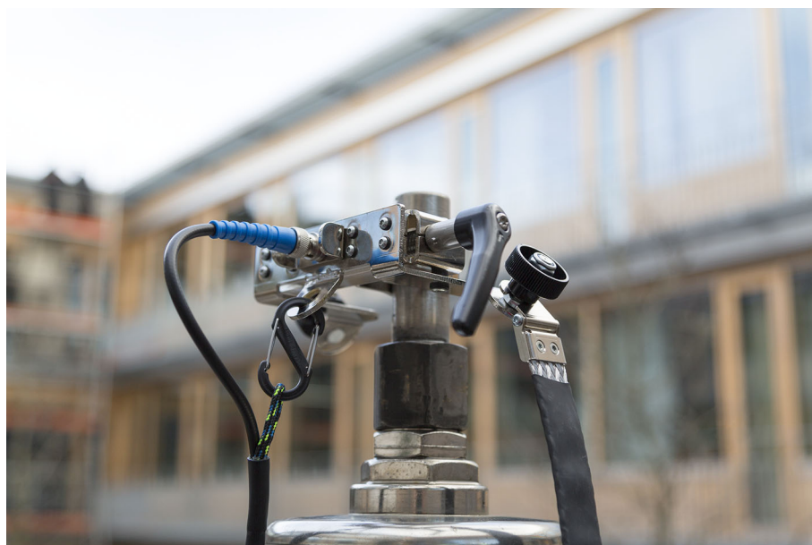
Figure 4-7: Connecting the blue coaxial cable to the bushing clamp by using the mechanism for relieving the pressure on the BNC shield
