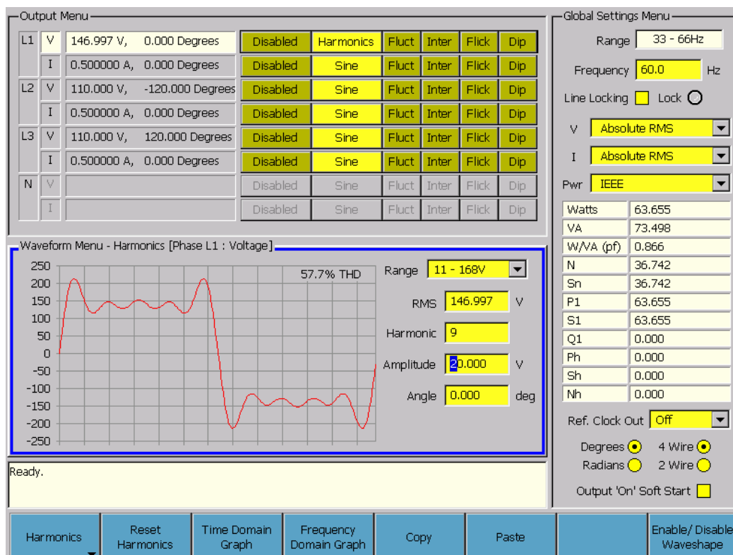
Figure 4-9. Harmonics with time domain graph
