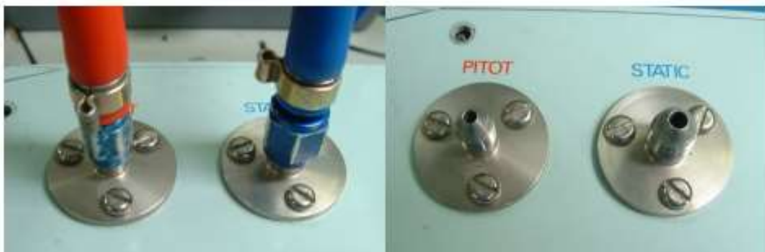
Figure 34 Distribution Unit's Input Connections and Inlets
