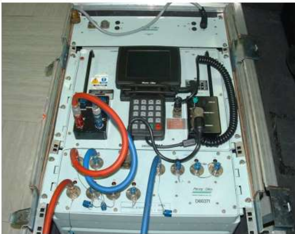
Figure 32 Connections between CCADTS 2 and Distribution Kit
