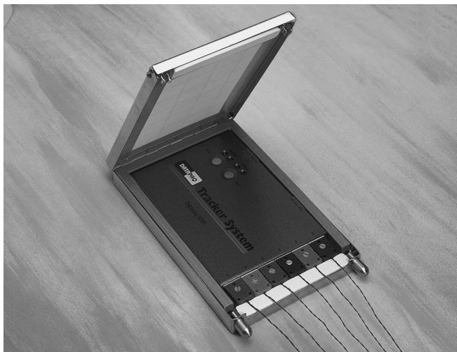
The logger in place in its thermal barrier.
