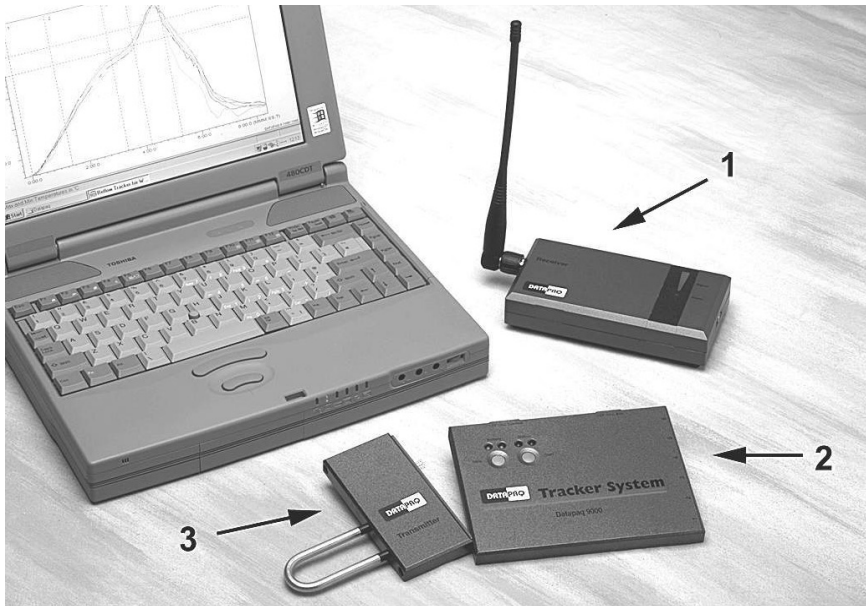
Radio-telemetry modules for Reflow Tracker. 1: Receiver 2: Datapaq 9000 data logger 3: Transmitter
