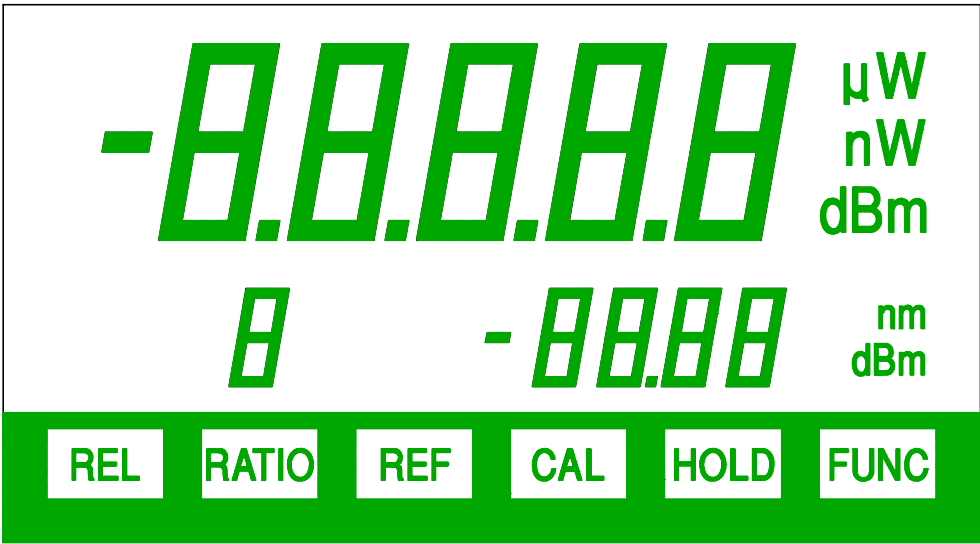
Figure 4-1 LCD segments and annunciators.
