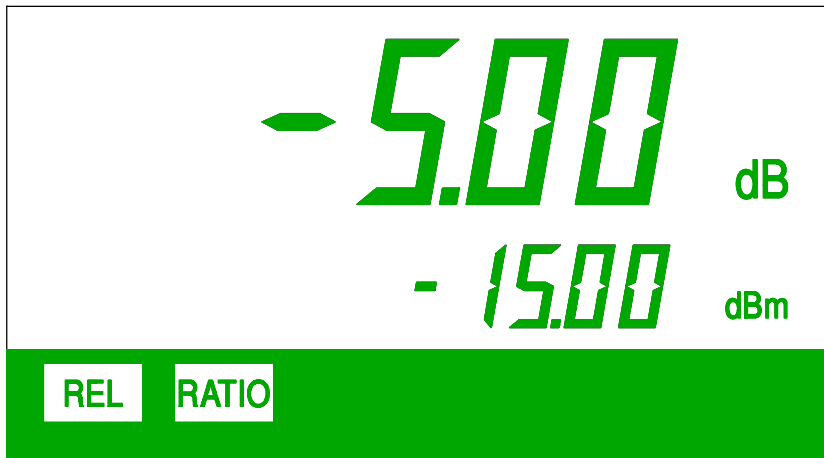
Figure 4-4 LCD display while in REL+RATIO mode.
