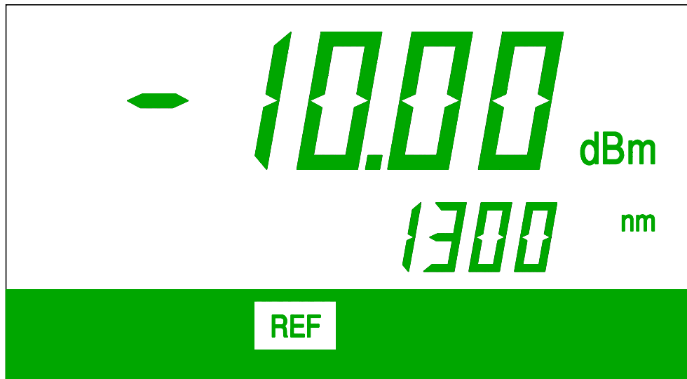
Figure 4-5 LCD display while in REF mode.
