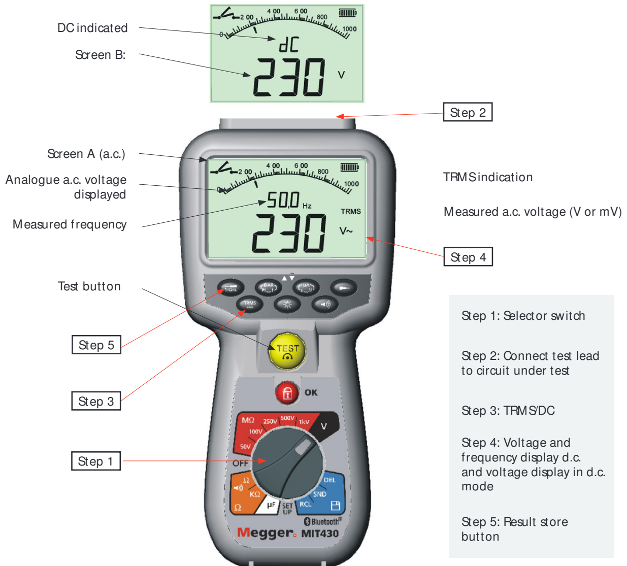
Figure 5 Voltage and frequency measurement
