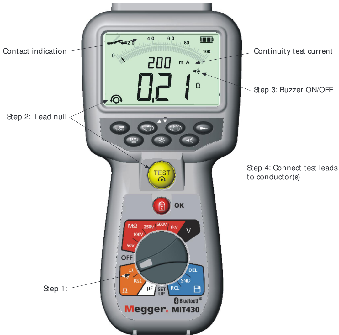
Figure 9 Continuity test and buzzer
