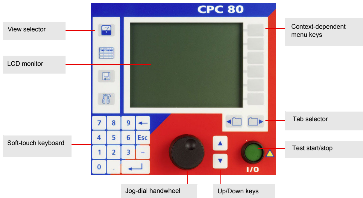
Figure 3-2: The CPC 80 's built-in ePC, components overview
