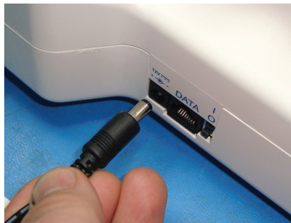
Figure 3-7 DC Power Plug
