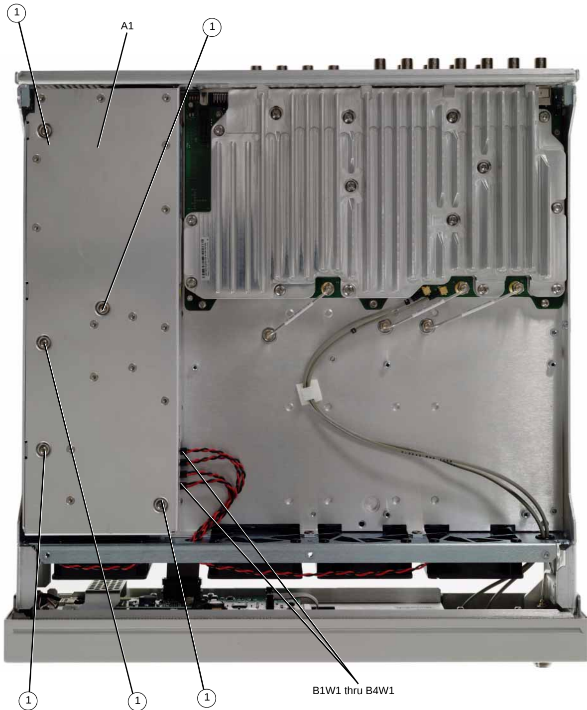
Figure 3-14 A1 Power Supply
