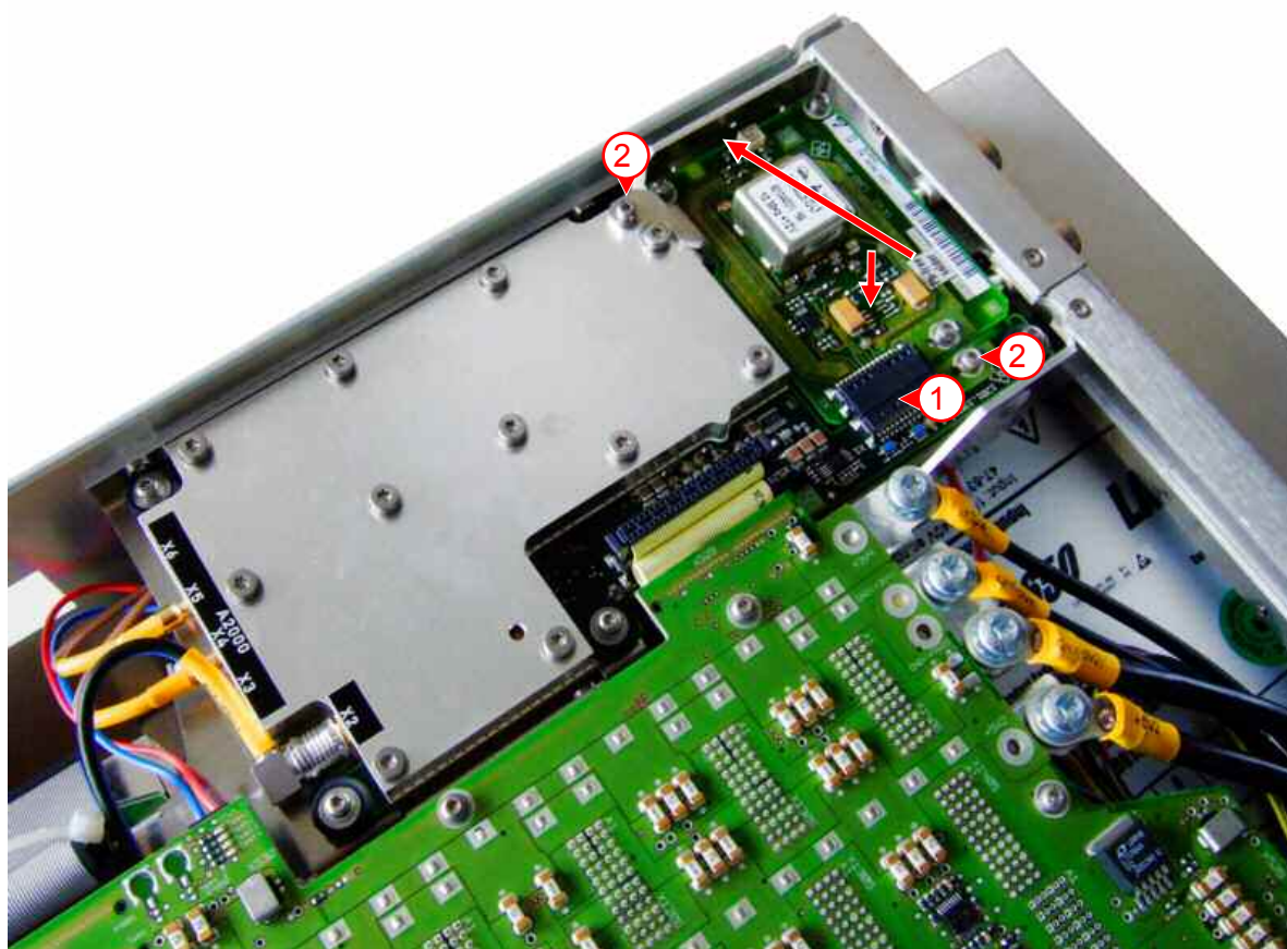
Figure 4 Mounting the OCXO MODULE
