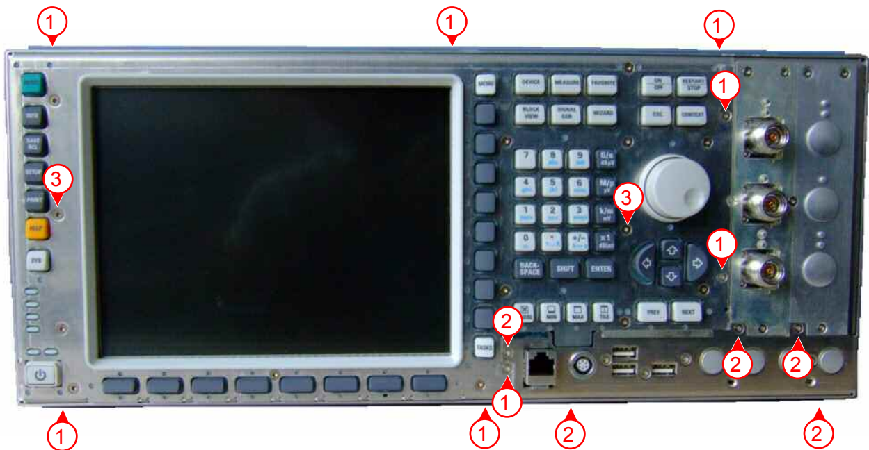
Figure 5 Removing the FP WITH MMI H600
