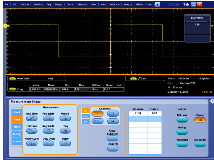
Figure 2-29: Measurement of probe compensator frequency
