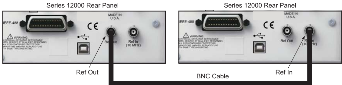
Figure 3-6 Ref Out and Ref In connections
