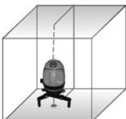
Front vertical and plumb point
