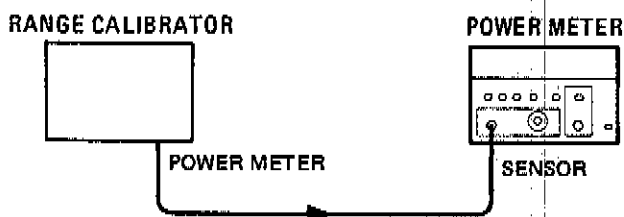
Figure 5-2. Auto Zero Offset Adjustment Setup
