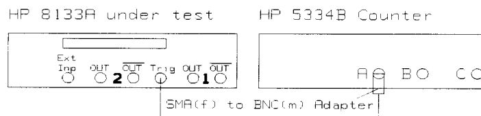
Figure 6-1. Internal Clock Low Frequency Test Set-up
